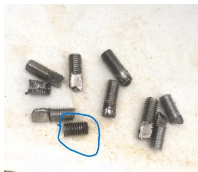
Pic 17; All 10 bolts removed from keel. Comment: The bottom part of all bolts, which are in the keel have treads as they were 'new'. Bolt with ring is most likely the bolt #8.
