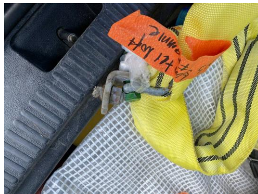
Pic 8b: Bolt # 4. Comment: Modified shackle and fiber sling replacing the original wire.
