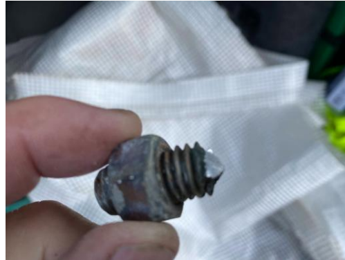
Pic 5b Bolt #1: Comment: A fresh cut shows the remaining strength of the bolt.
