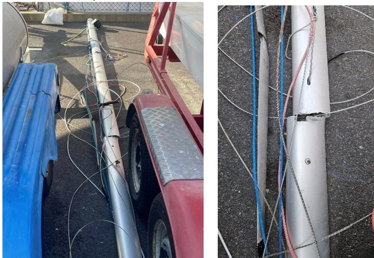
Pic 3 & 3b: Mast broken at the spreaders.
